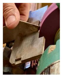
Nick brought along some A3 Sharpening guides for Skews, Scrapers and Gouges. The 3 files have already been copied and uploaded to the 'newsletter' page on the website so you can open and download and or save for reference. The Sorby pro-edge includes a set of recommended angle ranges on the machine.
