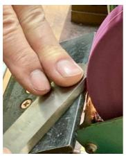
Tormek uses water to wet the stone – you must not leave the stone soaking in water or it will become out of balance. Equally, do not leave it wet in wintery conditions otherwise the stone may freeze and shatter.
