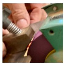
Never put a tool on the side of a grind stone – dangerous. Flatten the grind wheel profile with a dressing tool.
